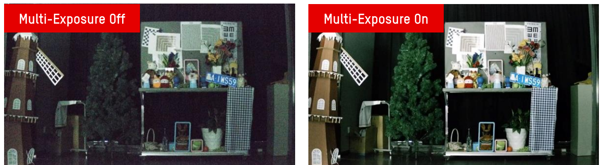
Figure 10 Multi-Exposure Off (Left) and On (Right)
