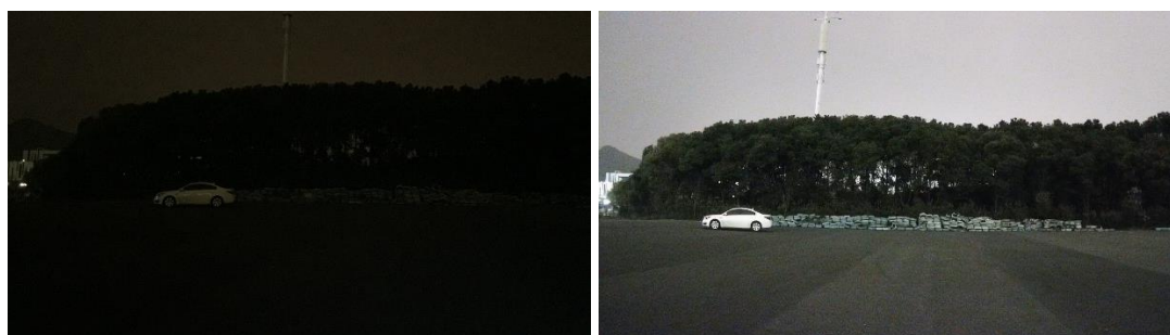
Figure 19 Photos Taken with iPhone 6s (Left) and DarkFighter Camera (Right)
