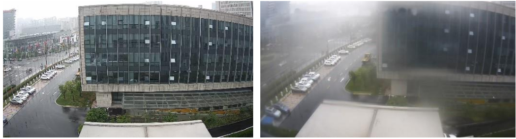
Figure 15 Camera Images with Anti-Fogging Glass (Left) and Normal Glass (Right)
