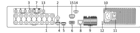
**NOTE** The rear panel of DS-7304/7308HQHI-K4 provides 4/8 video input interfaces.
